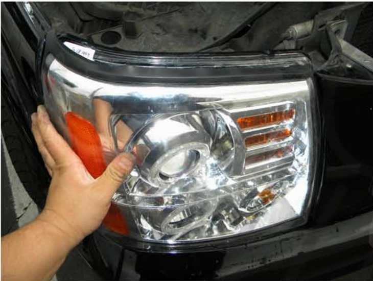
7. Install the new projector headlight
