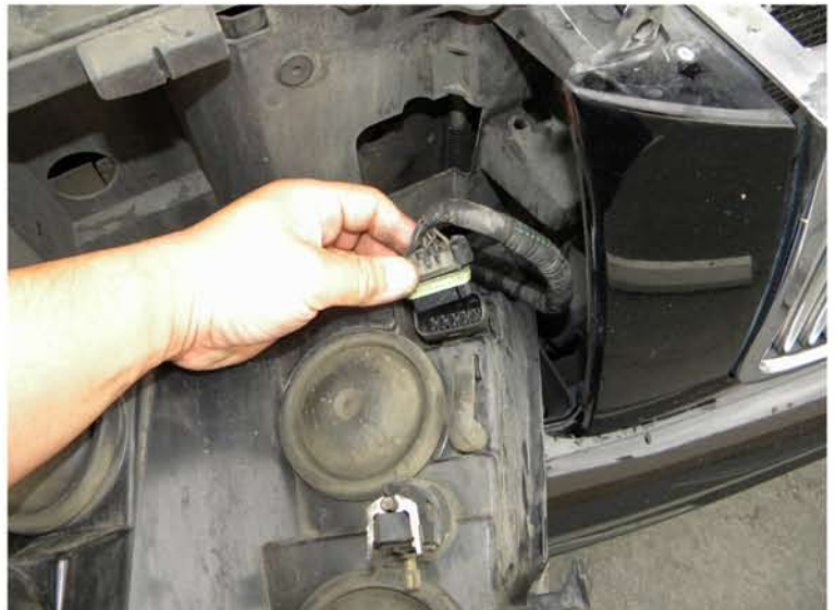
4. Disconnect the headlight harness
