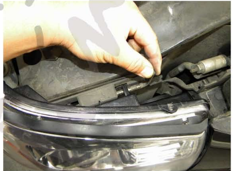
8. Put back the (2) lock Pins
