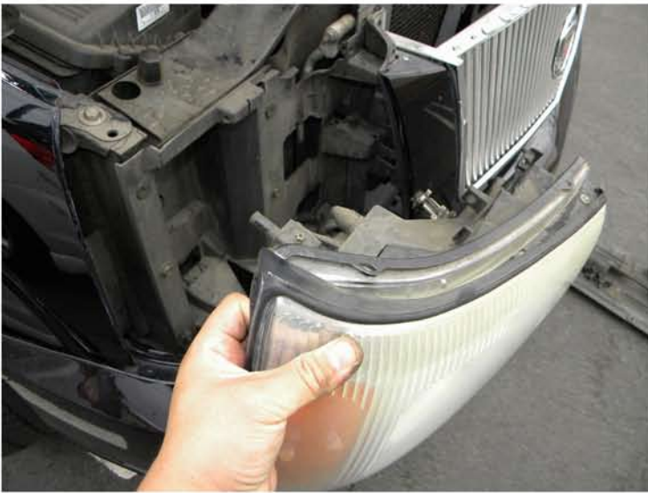
5. Remove the headlight
