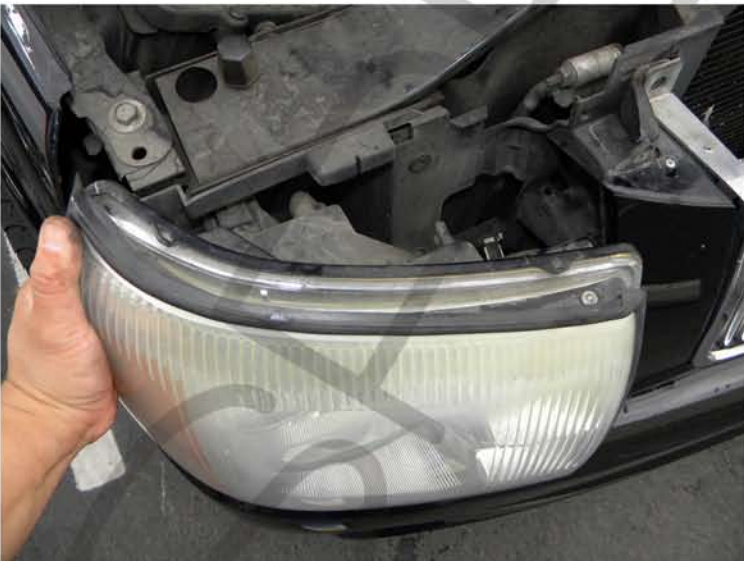
3. Pull out the headlight a little bit
